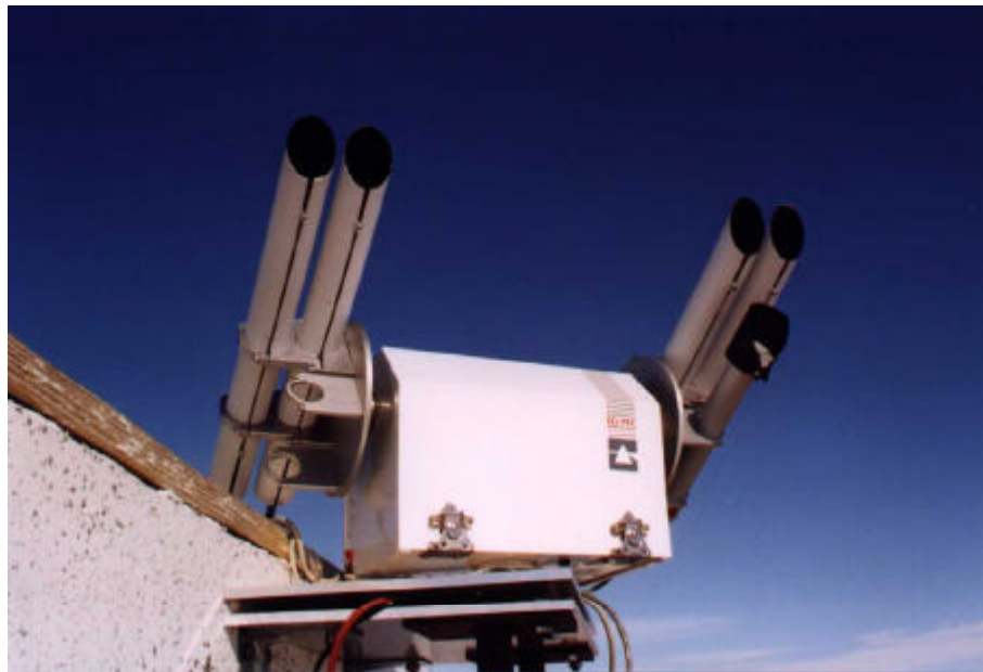
Figure 3.10: The photograph shows the four SolData pyrliometers (2M, 500, 1030 and 1550 nm) mounted within the climate shields, and the Kipp-Zonen 368 nm pyrliometer at the lower right.
