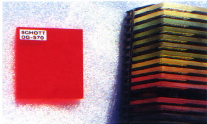
Figure 3.19: Schott high-pass filters transmit radiation above a specified cutoff wavelength.
