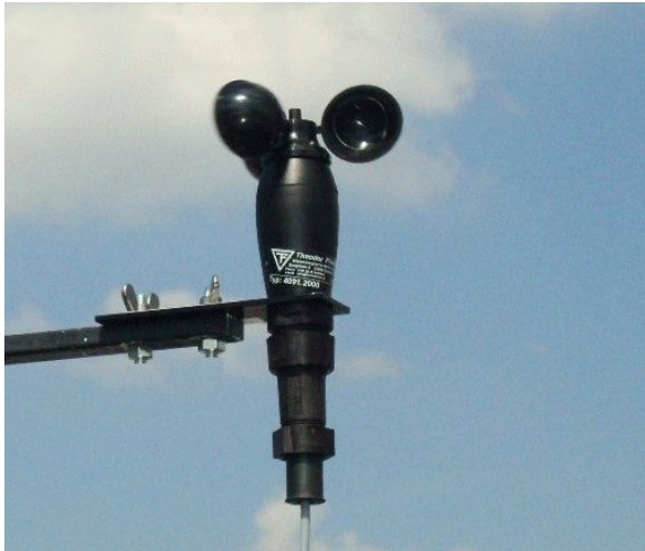
The SolData 110wss Wind Speed Sensor is manufactured by Th. Friedrichs in Germany.
