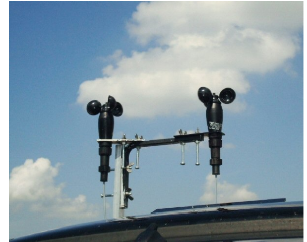
Calibration setup: test instrument and reference instrument are mounted on a moving vehicle.
