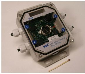
The HOBO U12-008 is weather resistant. It can collect data on 4 channels at the same time with 12 bit resolution.
