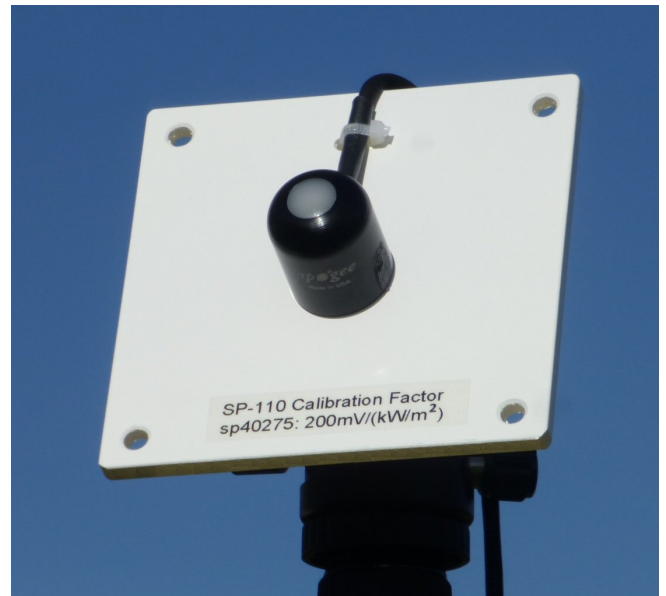
Figure 1: The Apogee SP-110 pyranometer is supplied with a 4.8 m cable.
