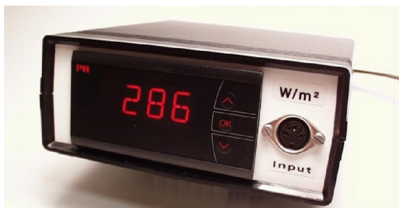
Figure 5: Continuous display of irradiance in W/m 2 can be achieved using a SolData DM-PYR. Options include relays and a 0-20mA current loop output signal.
