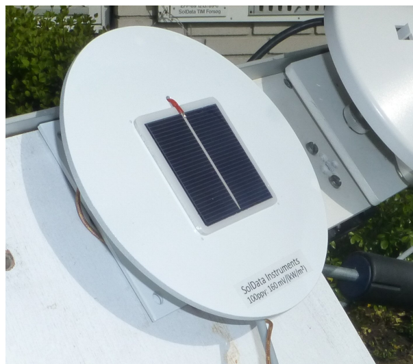
Figure 1: The SolData 114ppy pyranometer is supplied with a 3 meter long cable and a weather-proof IP54 connection to the instrument.
